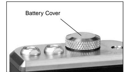
The TI-25LT is shipped with the batteries installed. Insert batteries in the polarity indicated on the rear label.
